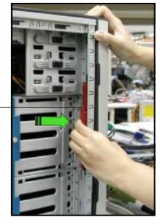
2. Pull and swing the left edge of the front panel outward.
